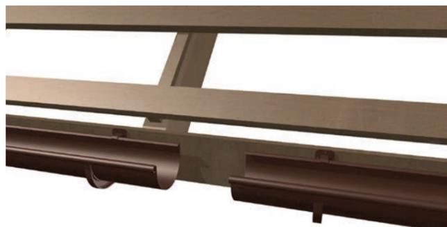
8. The drop outlet of the ProAqua system can be installed in two ways: as a pass-through or as a connector. In the first case, the appropriate hole diameter must be cut in the gutter, while in the second case, two sections of the gutter must be connected, following the recommendations of point 7.
